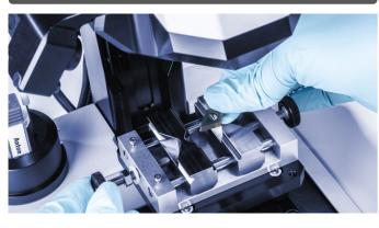
Start with the fused silica reference sample in the accessory kit with each instrument. Then mount your own sample.
