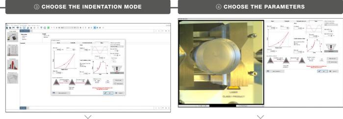
Choose between the 3 quasi static modes: linear, guadratic and constant strain-rate or the dynamic sinus mode. After choosing the mode, see the corresponding illustration of the indentation curve in the same window.
