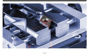
Now target the area to be measured with the laser. The indent is set at the intercept of the two laser lines. Add a camera, to more closely observe the area below.
