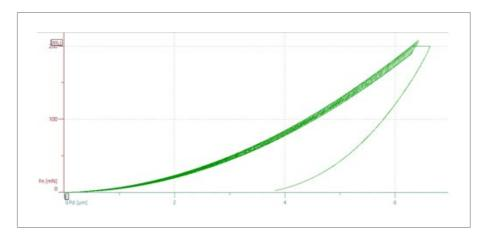
Figure 2: Typical indentation curve
