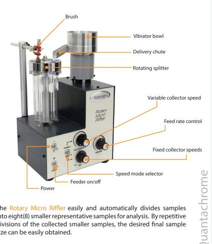
The Rotary Micro Riffler easily and automatically divides samples into eight(8) smaller representative samples for analysis. By repetitive divisions of the collected smaller samples, the desired final sample size can be easily obtained.
